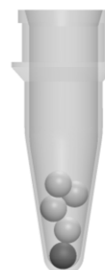
Figure 2: typical reaction contents with primers and intercalating dye lyophilised as beads in a typical 200µL PCR tube
