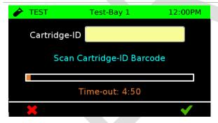
Enter Cartridge ID: scan the cartridge barcode or touch the yellow "Cartridge ID" field and manually type the barcode string using the alphanumeric on-screen keyboard. To get the barcode string, use a device with camera and barcode reading application (e.g. phone).
