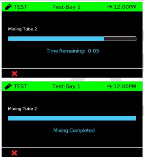
Wait 30 seconds for Tube 2 Mixing to complete by allowing the timer to elapse as shown on the screen. A double beep will sound when mixing is complete.
